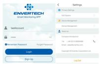
Step 2: Under "Device Management", click "Add" and enter MI SN manually or click the QR Code icon on the right to scan the MI SN automatically .
